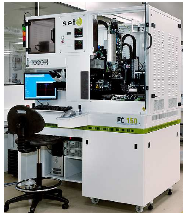
Fig.1 FC150 equipment by SET installed in the class 10 clean room at CNR-IMM, Catania
