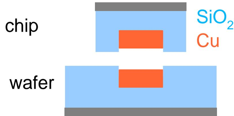
Damascene processing determines die and wafer surface topography.
