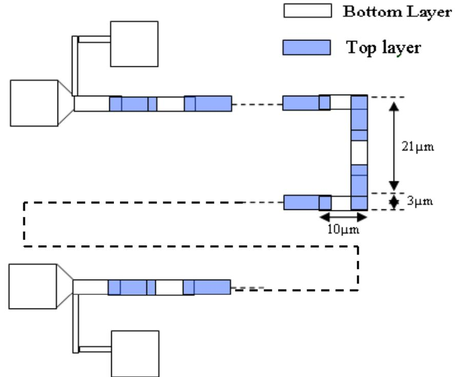
There are **10136** bonding contacts ( $3 \times 3 \mu\text{m}^2$ ) with  $7 \mu\text{m}$  pitch.
