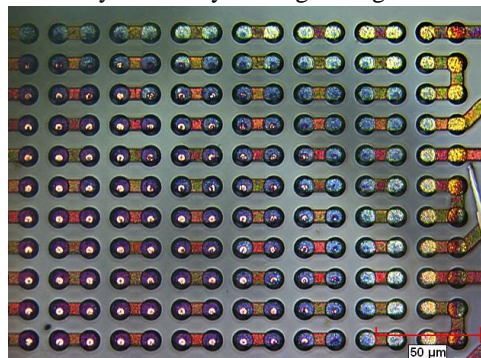
Fig. 16. CMP Cu – CMP Cu device after shear testing, showing oxidized bond pads along the edges and corner of the Plated Cu bottom die after shear testing.
