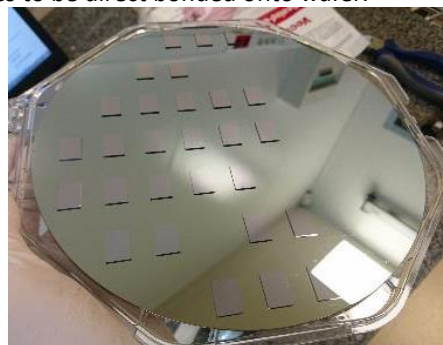
Chips direct bonded onto a Ø200 mm wafer on FC1 Beta tool at SET
