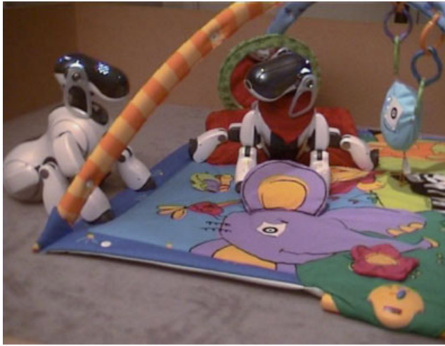
Figure 5. A four-legged robot is placed on a playmat. The robot can move its arms, its neck and its mouth, and can produce sound. Various toys are placed near the robot, as well as a pre-programmed 'adult' robot that can respond vocally to the other robot in certain conditions. This figure is available in colour online at www.interscience.wiley.com/journal/icd
