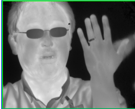
Figure 7. Broad-band LWIR image taken from the superlattice 320x256 Focal Plane Array using pixel substitution.
